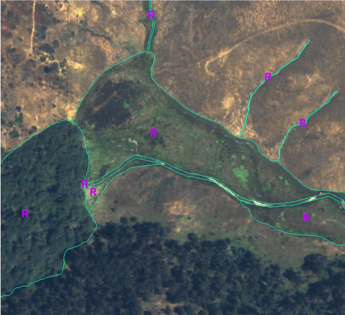
Figure C48: Channel with apparent channel and wide floodplain - If a channel's banks are apparent in the imagery, digitize the stream from bank to bank as a polygon in the wetland layer and attribute with appropriate channel classification.
