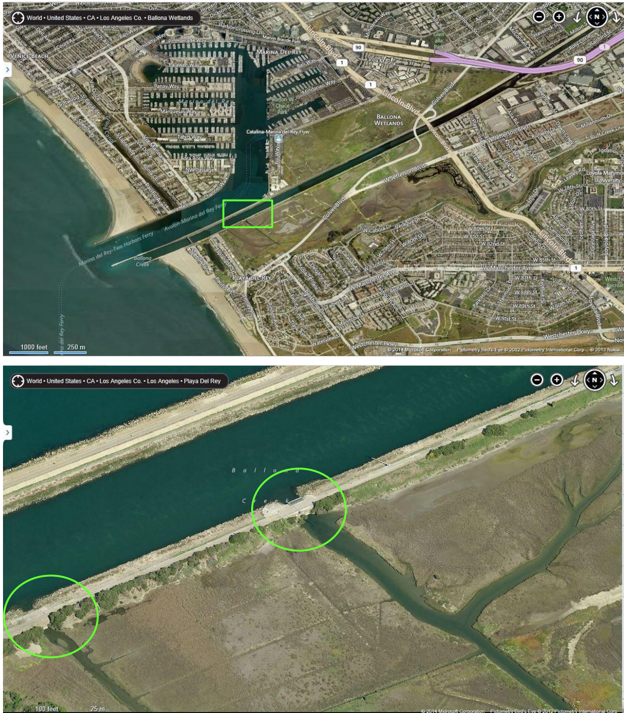
Figure C29: Ballona Wetlands, Southern California, example of estuary with muted tidal action (OE, WE). Culverts with flap gates allow limited amounts of sea water into the marsh via Ballona Creek (per CWIS). SoCal-specific.
