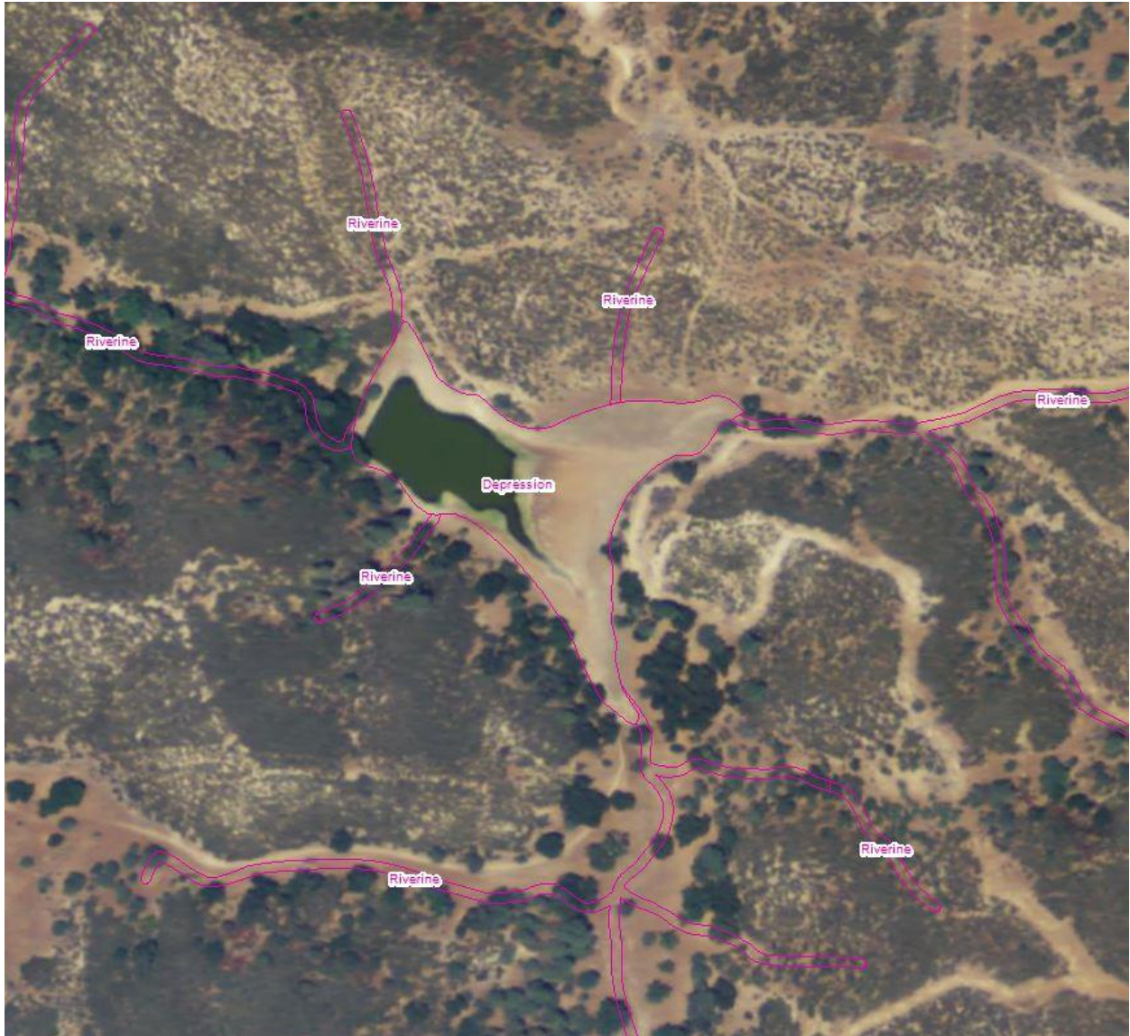
Figure C5: Delineate depressional wetlands (WD) to the visible outward extent of the draw-down zone, or OHW boundary.
