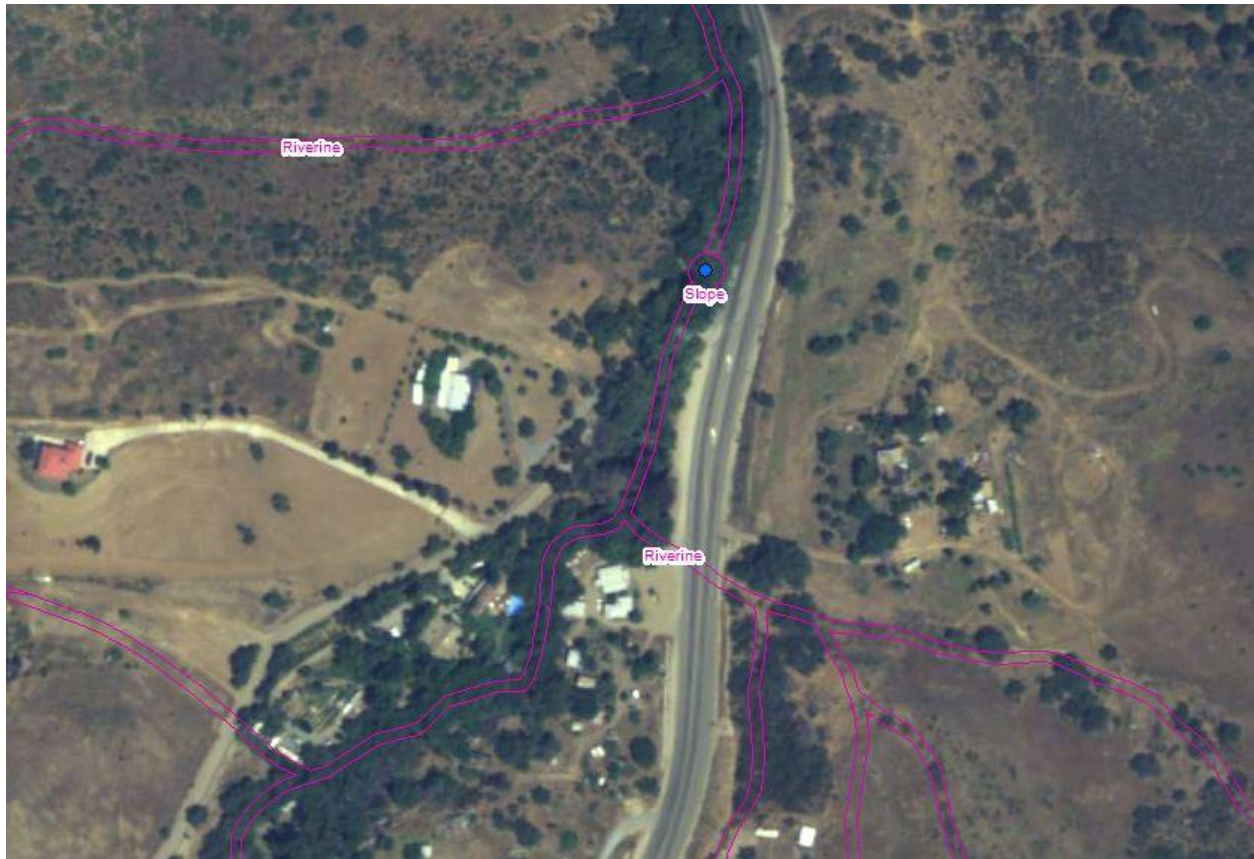
Figure C12: Check DRG and NHD datasets for springs that might not be visible on the imagery. If a spring exists in one of these two collateral datasets but is not visible in the imagery, buffer the point by 8 m and label as a slope wetland (WSs).
