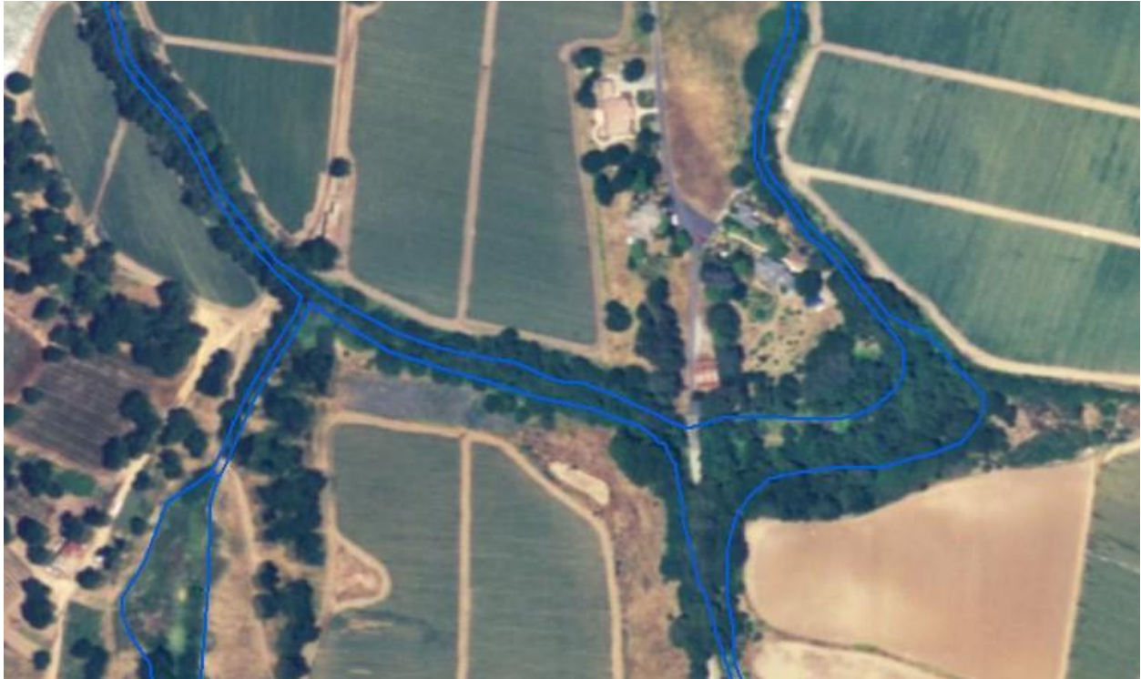
Figure C47: Channels with widening riparian area - Map the riparian vegetation when the DRG contours indicate a widening of the channel. Map only vegetation inside the banks of the riverine wetland.
