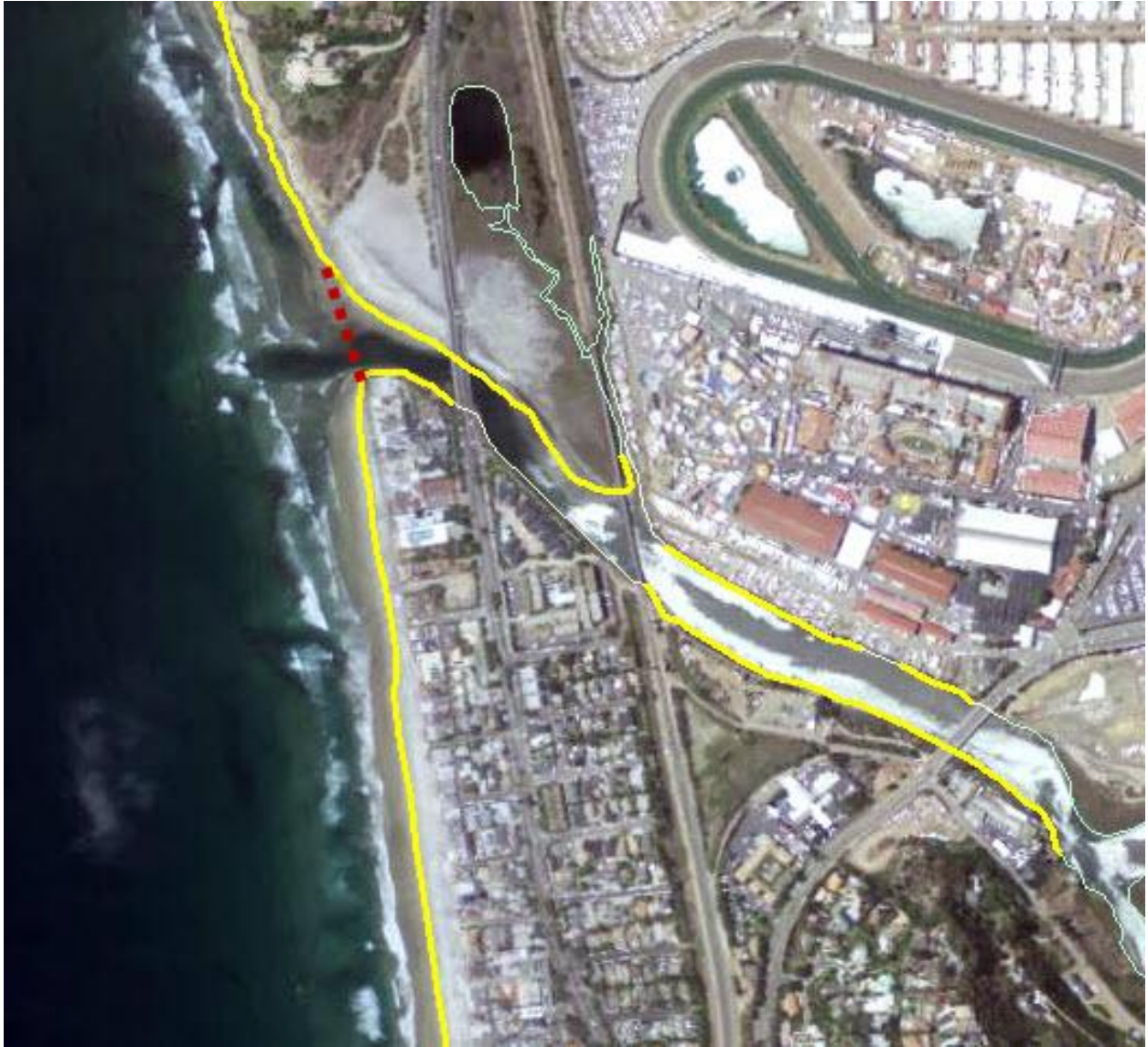
Figure C30: San Dieguito with the NOAA CUSP dataset MHW line. Division between estuarine area and marine area is made at the continuation of the shoreline across the mouth of the estuary.
