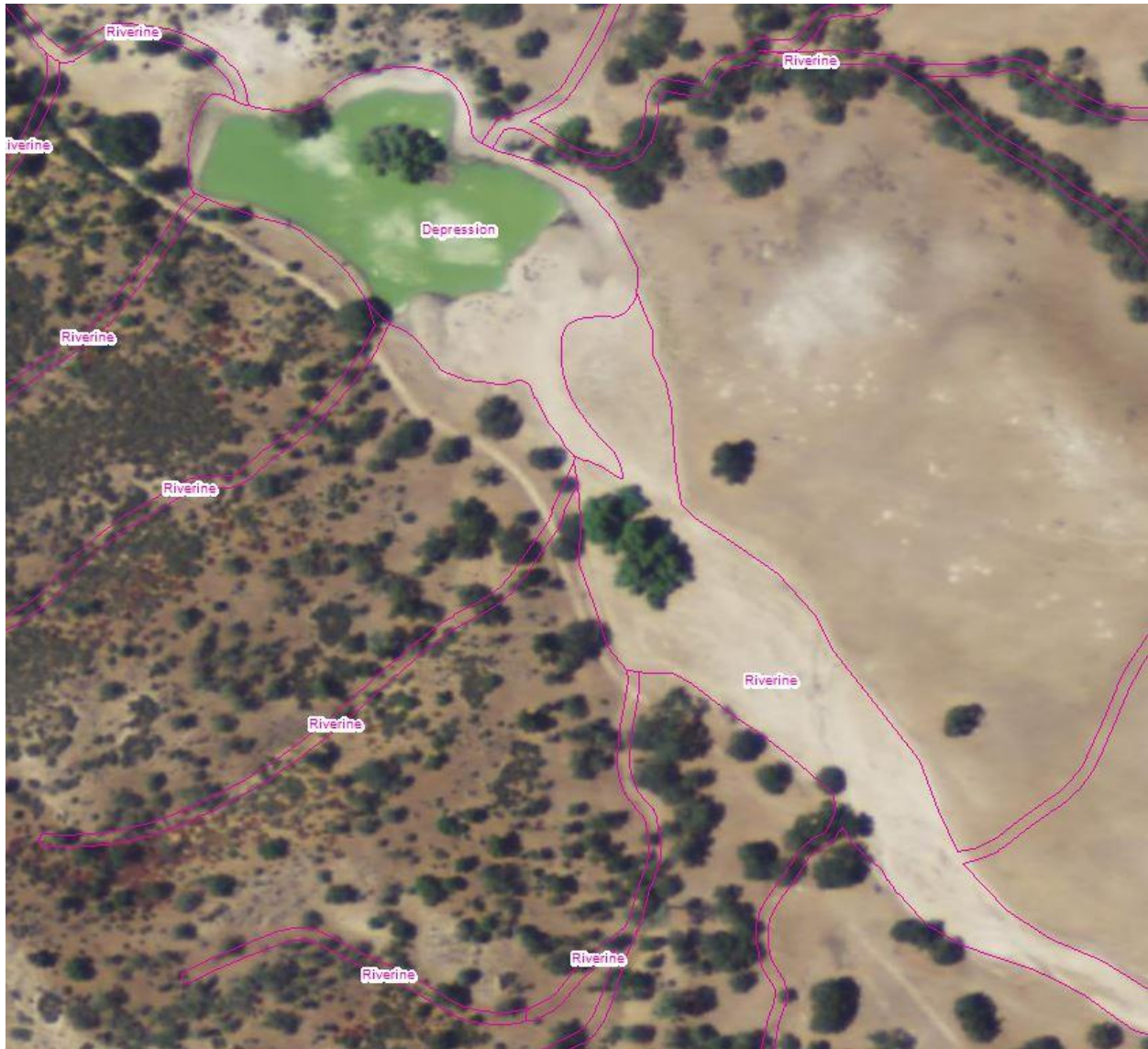
Figure C6: When a riverine feature is flowing into a depression, delineate the depression to the outward extent of the apparent drawdown zone.
