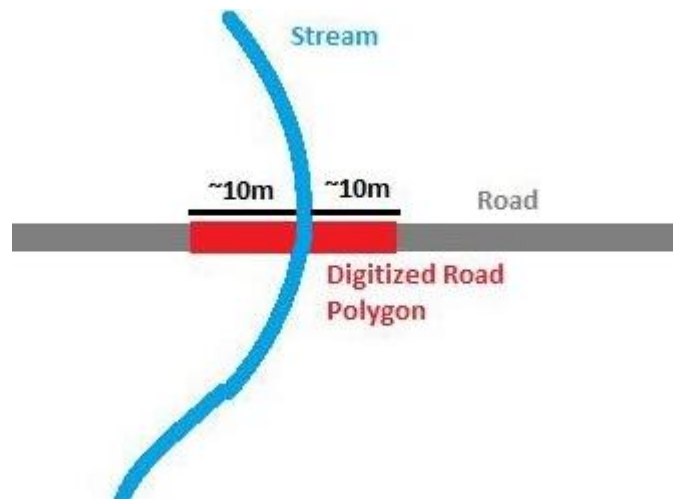
Figure 2. Illustration of mapping a road crossing over a stream, such as a bridge or culverted crossing. The stream (blue) is shown on top of the road (red) to indicate that it remains a contiguous feature that flows under the road. If the road was paved in the stream (e.g., a dip/Arizona crossing), the road (red) would be shown on top to indicate a break in the continuity of the stream.
